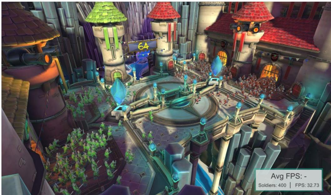
When building levels, try to keep overdraw to a minimum. Unity lets you measure and visualize the amount of overdraw that is in a scene. This mode is highlighted in the following screenshot:
